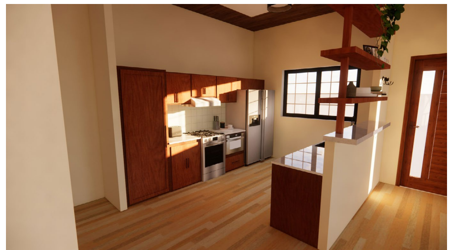
Shelves and counter tops are lower than normal to accommodate someone in a wheelchair or who is unable to reach higher up. Cabinets use easy-to pull and grab handles.
